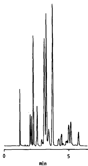
Fig. 12. Chromatogram of a gasoline. TCD, type II, 68°C, 15 Torr. Column B, 68°C. Sample size, 0.1 μl; splitting ratio, 1:50.
